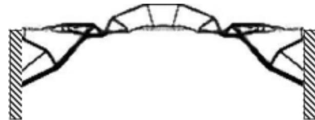
maximizing the minimum buckling load
