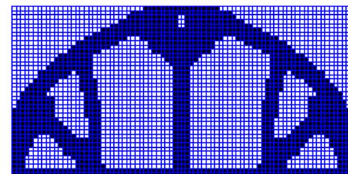
b) filtered design without checkerboarding.
