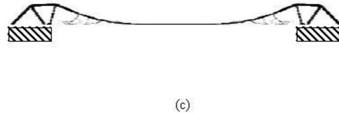
**Design to maximize minimum linearized buckling eigenvalue**
