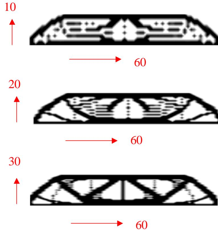
Cure with mesh refinement in direction of layering.
